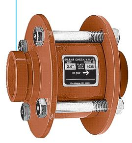
The 400G is a center guided, spring loaded, silent check valve. Designed and engineered for silent operation with low head loss, the valve disc will close prior to the reversal of flow, thereby preventing or minimizing water hammer and damaging shock.
